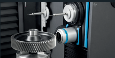
Pitch measurement on cylindrical gears
