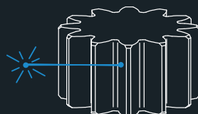
Pitch measurement on cylindrical gears
