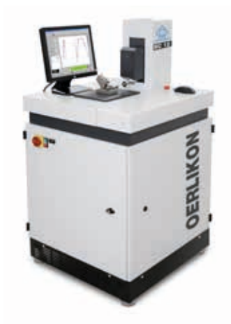
Oerlikon stick blade measuring device BC 12 for high-precision measuring of stick blades and documenting the individual blades
